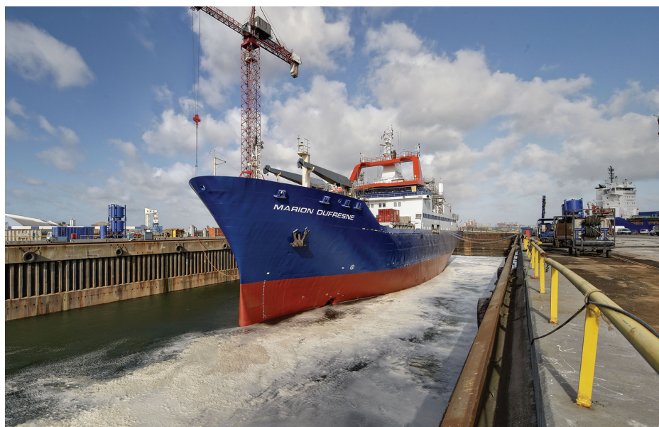
Figure 1: Research Vessel Marion Dufresne in dry dock during her complete refit (photo by Damen Shiprepair Dunkerque).
