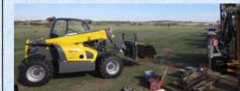
Compact telehandler: Operating weight = 2.55T, max payload = 1.2T, max range = 2.29m, payload for max range = 0.44T.
