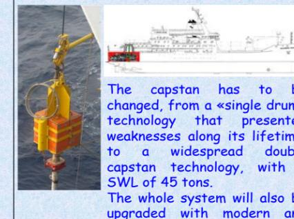
The capstan has to be changed, from a «single drum» technology that presented weaknesses along its lifetime, to a widespread double capstan technology, with a SWL of 45 tons. The whole system will also be upgraded with modern and more reliable technologies.
