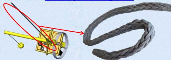
A new 7000 metres oceanographic cable will be designed to fit with the new requirements of «perfect» long coring: it has to be both extremely strong - to bear 45 tons extraction strength of giant pipes - and very stiff. New fibers and braidings are under investigation and development.
